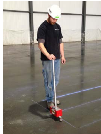
Figure 2: Slab profiling instrument
