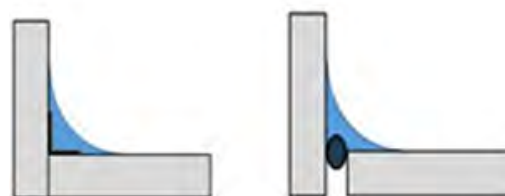
Image 2: Tight inside corner joints
