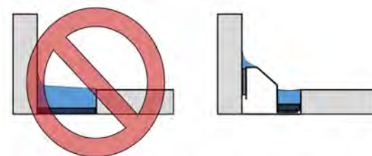
Image 3: Wide inside corner joints
