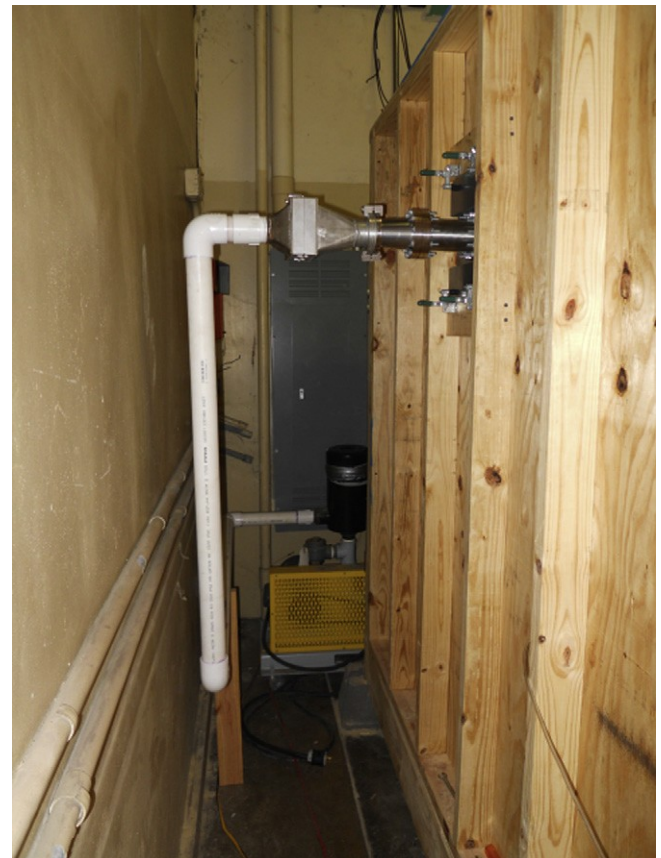
Fig. 3. Outlet system e showing outlet tube to filter to vacuum pump.
