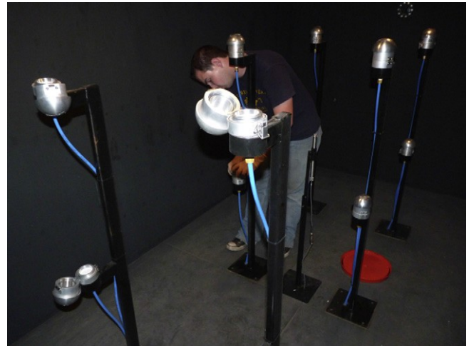
Fig. 4. Room particulate sampler system \phi 12 samplers at two heights, three depths, and two cross-section locations.
