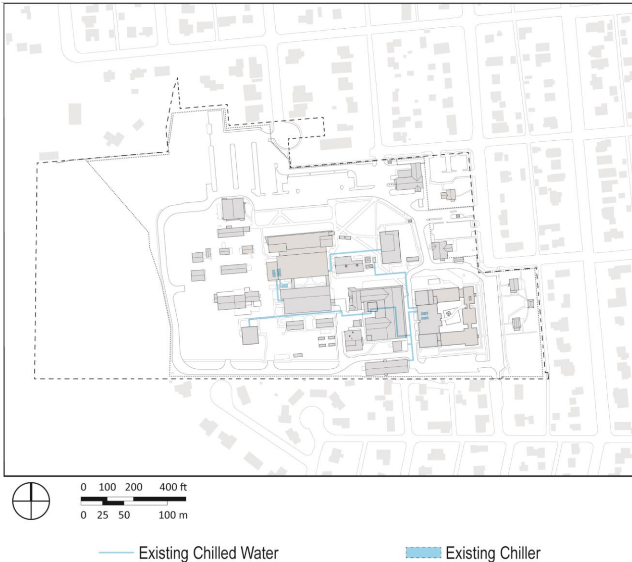
Exhibit 3-30: Existing Chilled Water Plant
