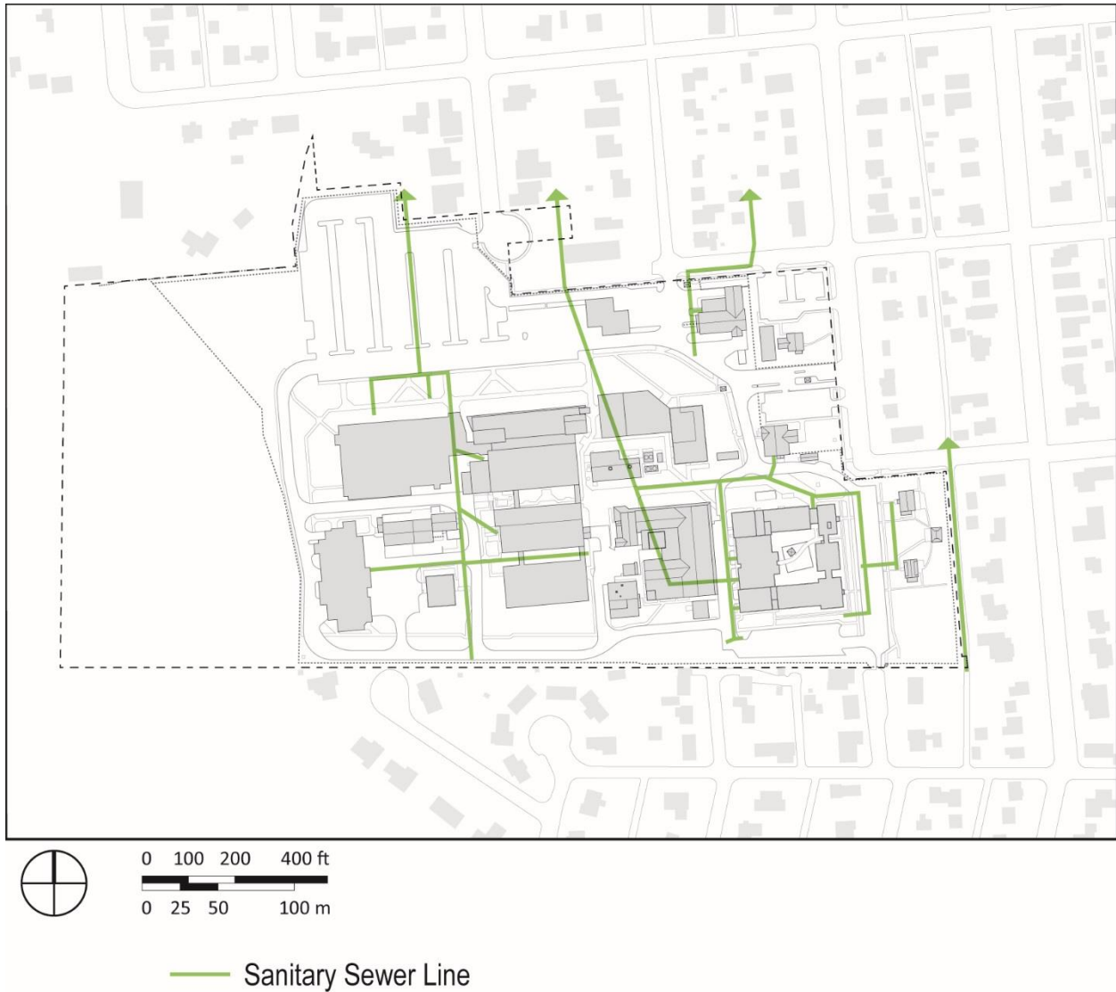
Exhibit 4-26: Projected Sanitary Sewer
