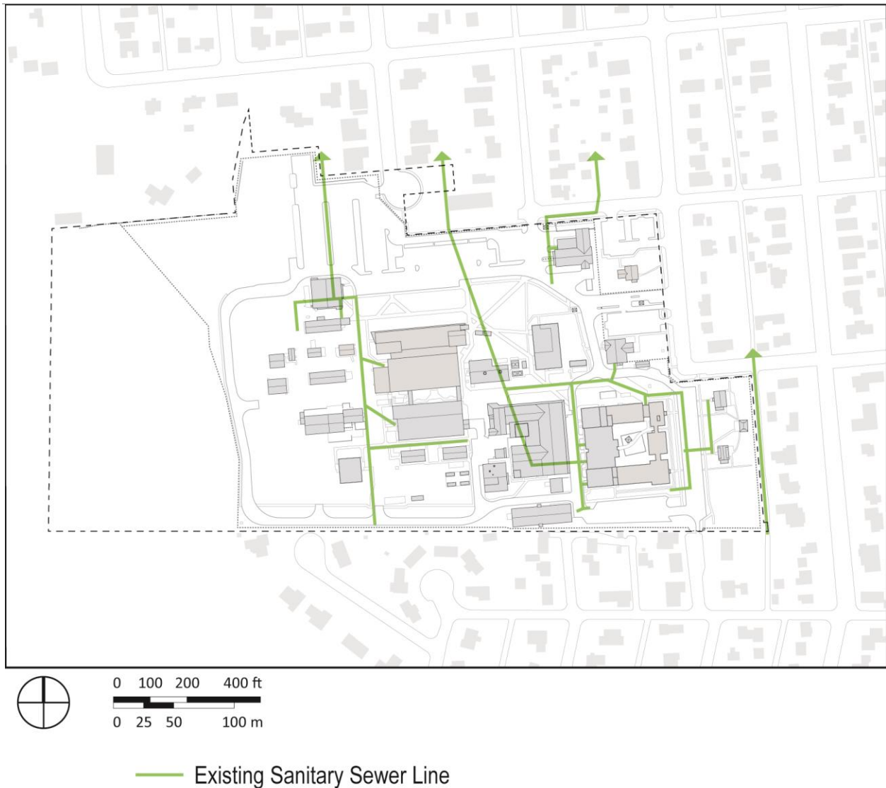
Exhibit 3-34: Existing Sanitary Sewer
