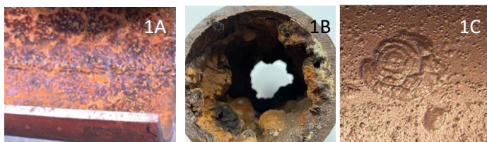
Figure 1: Steel pipe corrosion due to DO levels (1A), tuberculation (1B), and MIC (1C). [cibsejournal.com, NIH DTR, and escorrosion.com]
