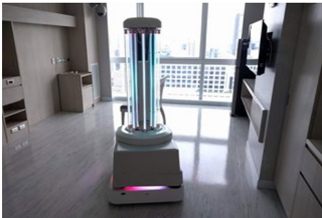
Figure 2 – Robotized UV Disinfection
