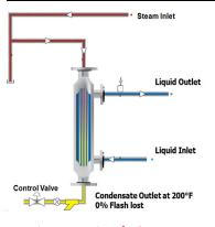
Figure 1 Basics of a Steam Domestic Water Heater <sup>(1)</sup>
