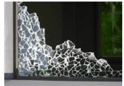
Figure 2: shattered tempered glass
