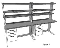
characteristics are most useful, including wet areas, areas requiring heavy loading and stable work platforms, and areas not likely to change function. Install flexible benches in 'dry' areas, areas of lighter duty, and areas likely to be reconfigured.
