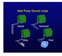
inserted before the hole is backfilled. Each vertical pipe is then connected to horizontal underground pipe that carries fluid in a closed system to and from the indoor exchange unit. Vertical loops are generally more expensive to install, but require less piping than horizontal loops because the earth's temperature is more stable farther below the surface.
