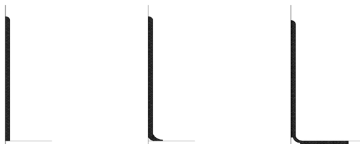
Types of Resilient Bases: Straight, Cove, Sanitary Toe
