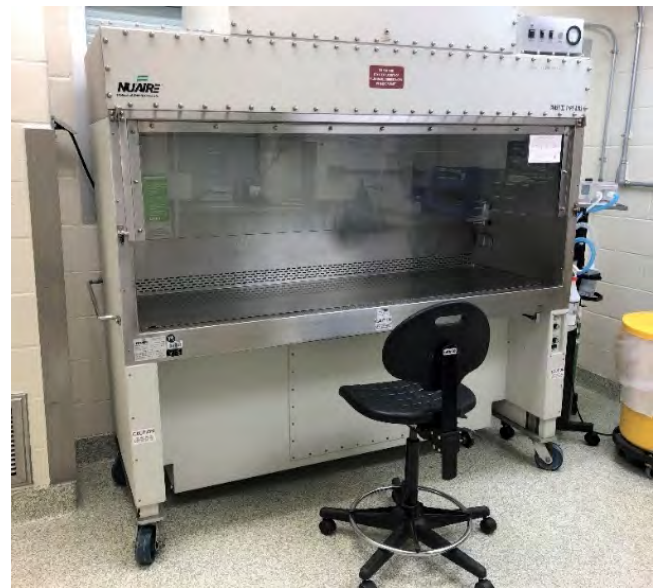
Figure 2.3.4.4: Animal transfer station example, non-ducted
