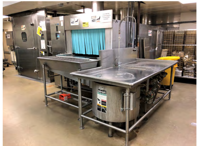
4.6.2.1.A.2: Tunnel washer with dump station and waste disposal system (Credit NIH OD/ORS/Division of Veterinary Resources)
