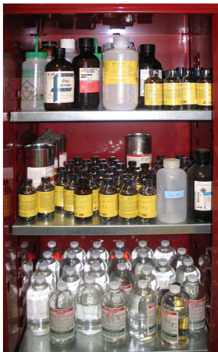
Figure 4.5.3.2: Flammable storage cabinet
