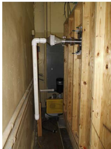
Fig. 2. Front view of testing chamber with air inlet pipe (top). The outlet system in the back view (bottom) contains a glass fiber filter and connects to a vacuum pump.
