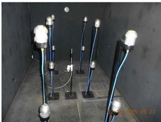
Fig. 3. The nebulizer (top) and air samplers (bottom) installed in the testing chamber to suspend the particles and collect them, respectively.
